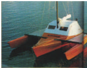
Above: The canopy completely encloses the cockpit. There is room for eight adults to sit in the cockpit in comfort
